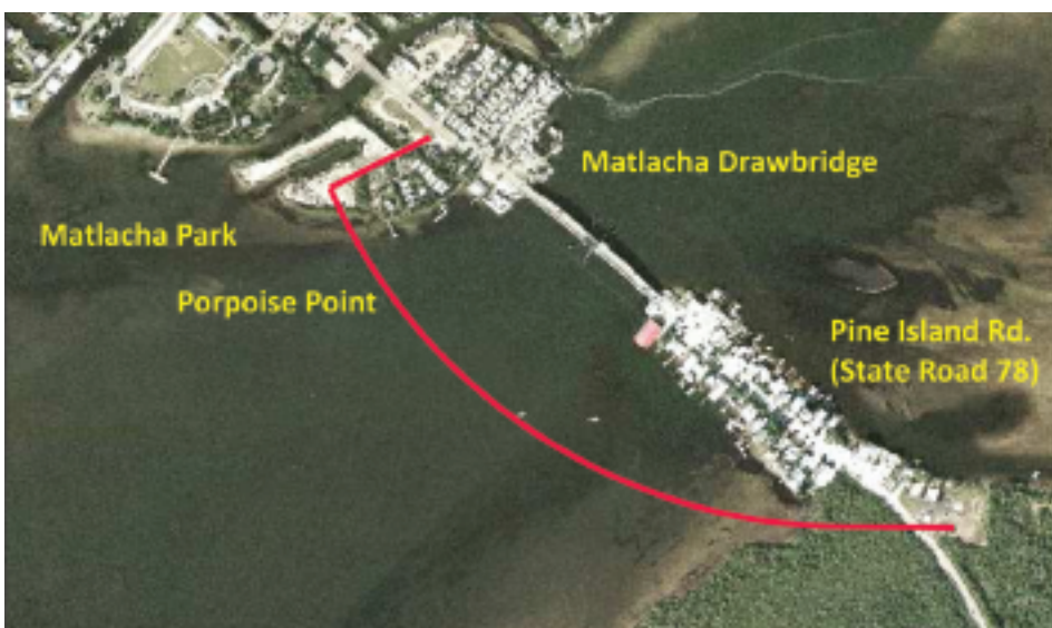
Figure 4 - Alternate Pipe Route 3 Selected
